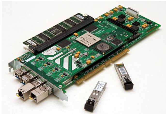
Fig. 2. FlowMon - COMBO6X PCI-X 64/66MHz hardware accelerated card [14]
