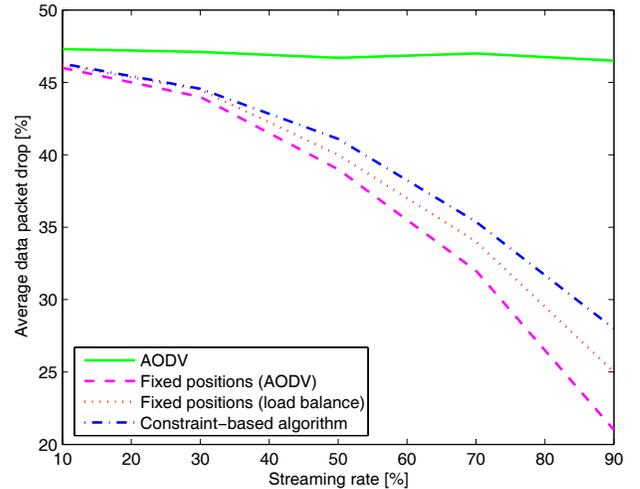
Fig. 2. Dependency of packet drop on streaming rate
